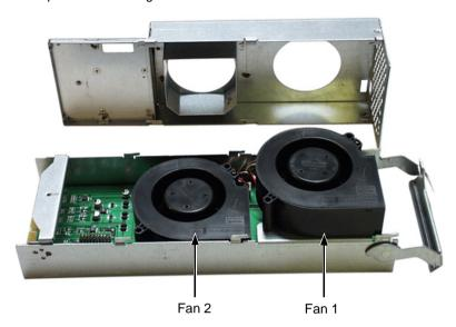
The upper fan is Fan 1, the lower fan is Fan 2. From the LEDs on the cooling unit (see the diagram on page 221), you know which fan to replace.
